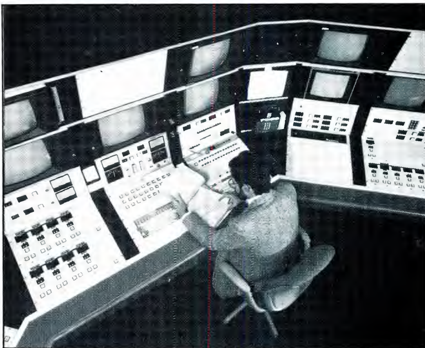
Satellite distribution systems have provided expanded flexibility for radio networks. The number of networks offering programming of various types also has increased. Shown is the switching control center of ABC Radio in New York. (Courtesy of ABC.)
