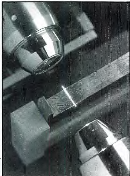
Through non-linear optics techniques, this small piece of fiber can self-switch an input to one of two output paths, based on the power of the input pulse.
